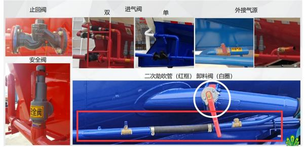
**3.** 高端罐体焊接工艺, 罐体内加装加强圈和横向支撑, 双安全泄压阀设计, 加装压力指示仪表, 罐体承压性和安全性更高 High-end tank body welding process, reinforcement ring and lateral support are installed inside the tank body, double safety relief valve design, installation of pressure indicator, the tank body has higher pressure bearing and more safety;
