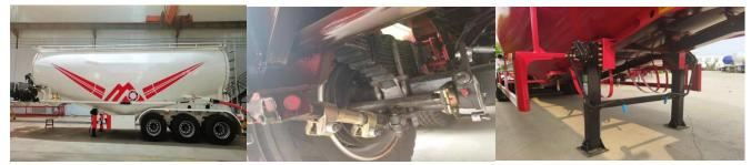
2. 罐体结构优化,适用多种运输介质,出料口加装二次助吹结构, 卸货速度更快,卸货残余量将至最低 The tank structure is optimized, suitable various bulk cement cargoes, the discharge pipe is equipped with a secondary blowing-assisting pipe, which makes the unloading speed faster and the residual amount of unloading will be minimized.;
